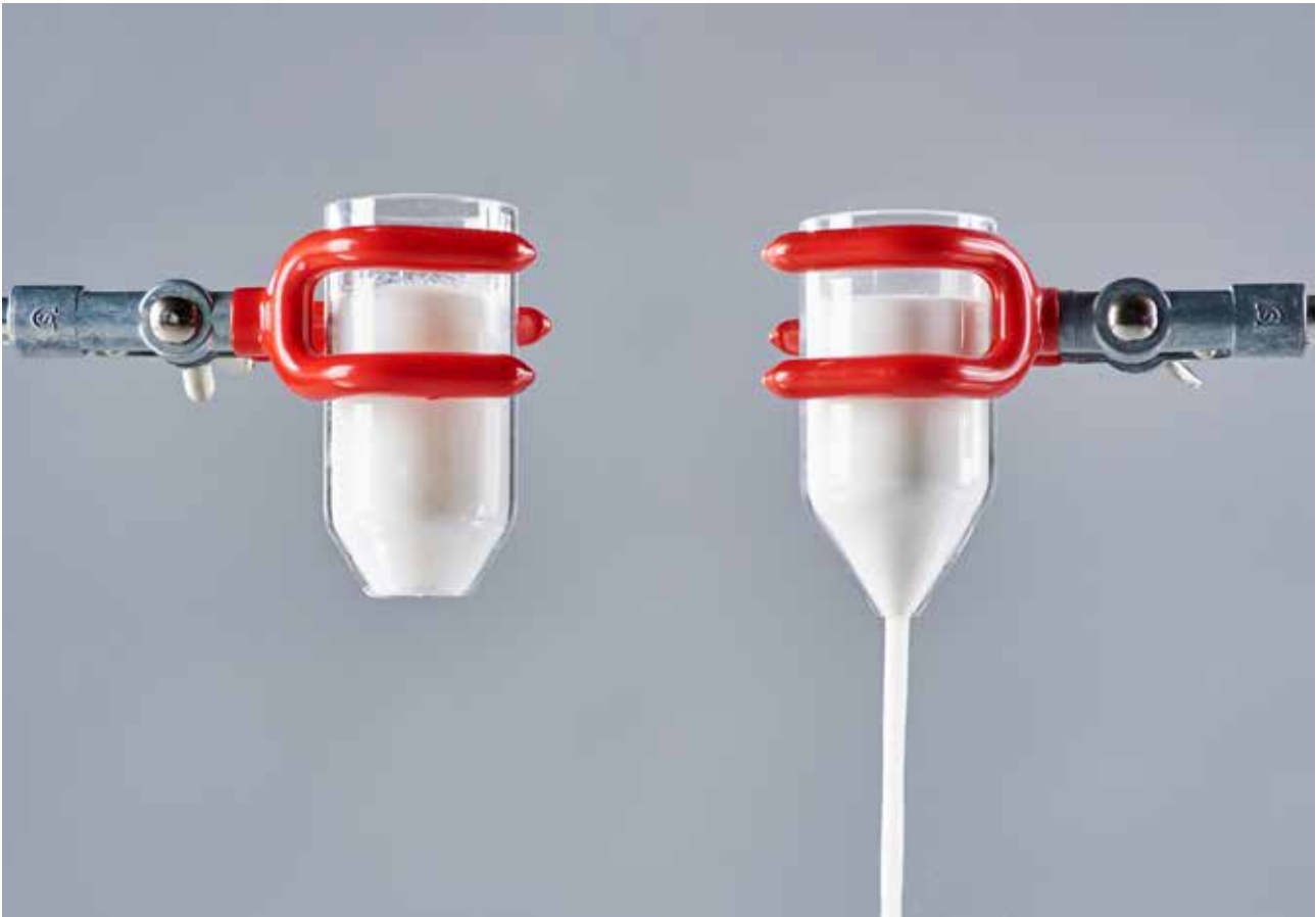
Figure 4: Flow properties of AEROSIL® 300 (left) and AEROPERL® 300 Pharma (right)
