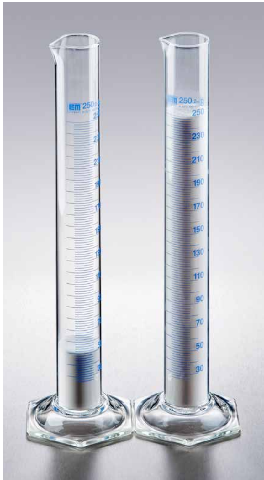
Figure 5: Difference in tamped densities between AEROPERL® 300 Pharma (left) and AEROSIL® 300 (right) — both cylinders contain the same weight of material.
