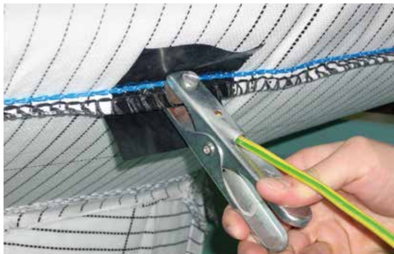
Figure 3 Grounding of an FIBC
