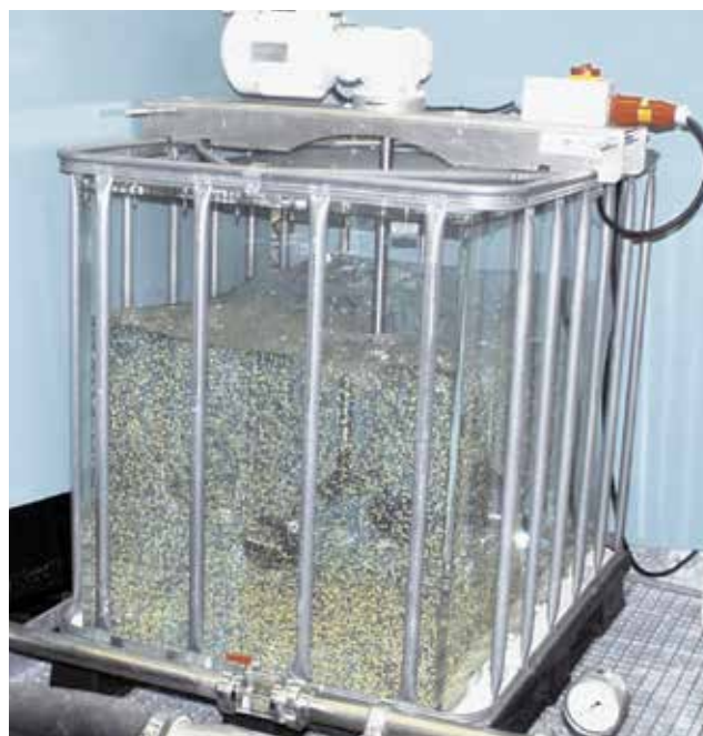
Figure 11 Viscojet during dispersion process
