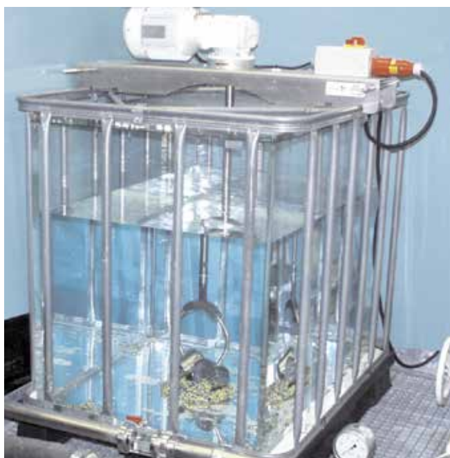
Figure 10 Viscojet in IBC prior to dispersion
