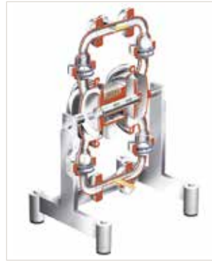
Figure 12 Double membrane pumps
