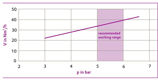
This means that 39 Nm³/h of air at 6 bar is to be provided during the fluidization pulse. However, for example with fluidization of 1 second pulse and 9 seconds pause, the resulting air consumption is just 3.9 Nm³/h. To actually provide this air volume on the PESy during the short pulse, the solenoid valve and the feed hose must not be too small. An inner diameter of 12 mm has proven to be suitable. The distance between the solenoid valve and the PESy should also not exceed 5 meters.
