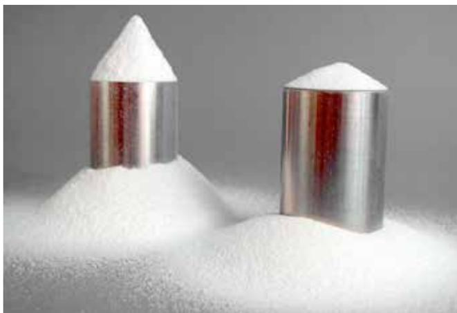
**Figure 1** The cone height indicates bad (left) or good (right) flowability
