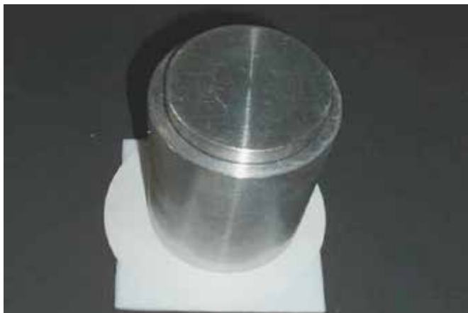
Figure 8 Steel cylinder on a filter paper to determine absorption capacity
