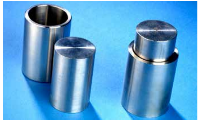
Figure 6 Steel cylinder to determine caking tendency
