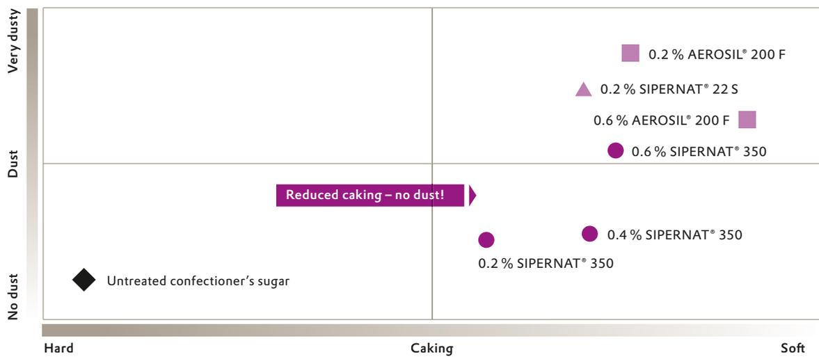
Confectioner's sugar (particle size between 50 – 100 µm) treated with corresponding silica, dosage given as wt%; mixing in lab mixer (Somakon) with varying duration at 2000 rpm to simulate milling
