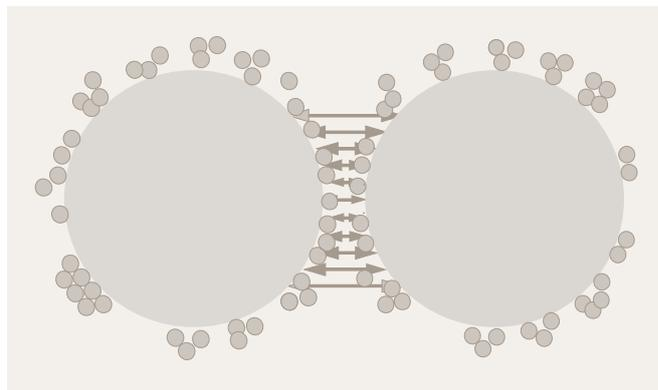
Figure 2 AEROSIL® fumed silica resp. SIPERNAT® specialty silica cover the host powder's surface and act as a spacer
