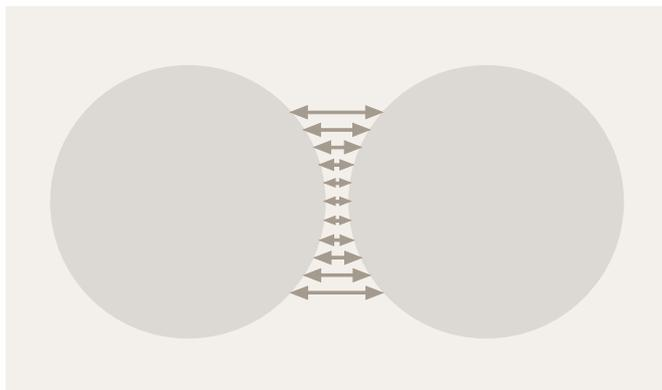
Figure 1 Particles sticking together by Van-der-Waals forces
