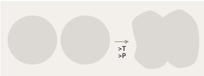
**Figure 3** Soft or thermoplastic particles stick together as they are deformed on pressure and rising temperature
