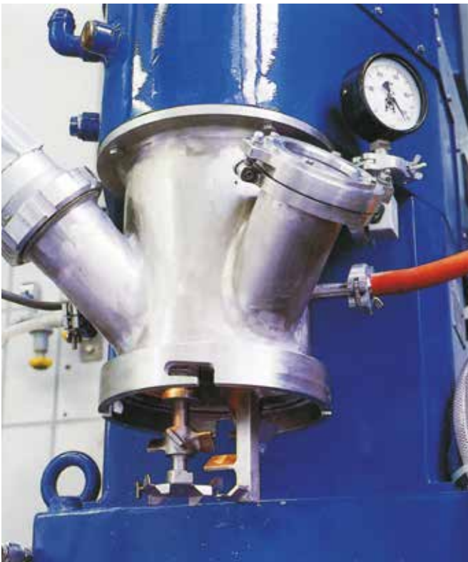
Figure 15 Lab planetary dissolver with vacuum- and inert gas equipment (Hermann Linden GmbH & Co., KG, D-51709, Marienheide, Germany).
