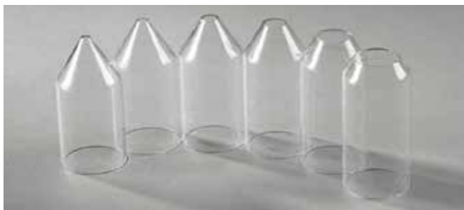
Figure 2 Set of glass funnels for measuring the flowability
