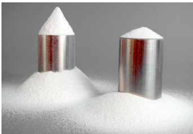
Figure 1 The cone height indicates bad (left) or good (right) flowability
